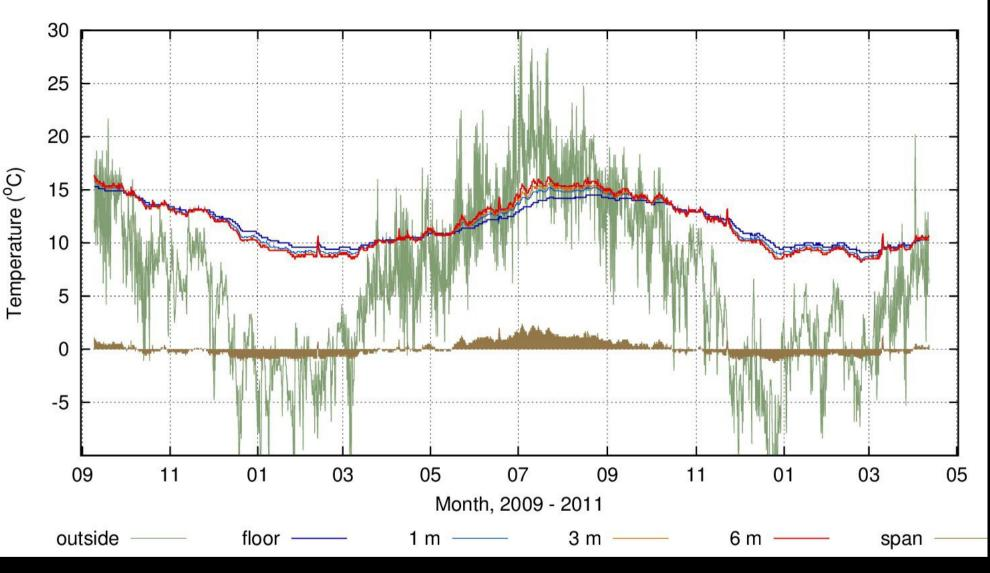
The annual temperature cycle at various heights within the museum store in Ribe. The annual cycle span is reduced to 8 K. There is very little temperature stratification The following ranges of RH and temperature are recommended as a means of preventing even sensitive archival materials referred to within **4.2.2** from being compromised when stored alongside less critically sensitive archival material:
