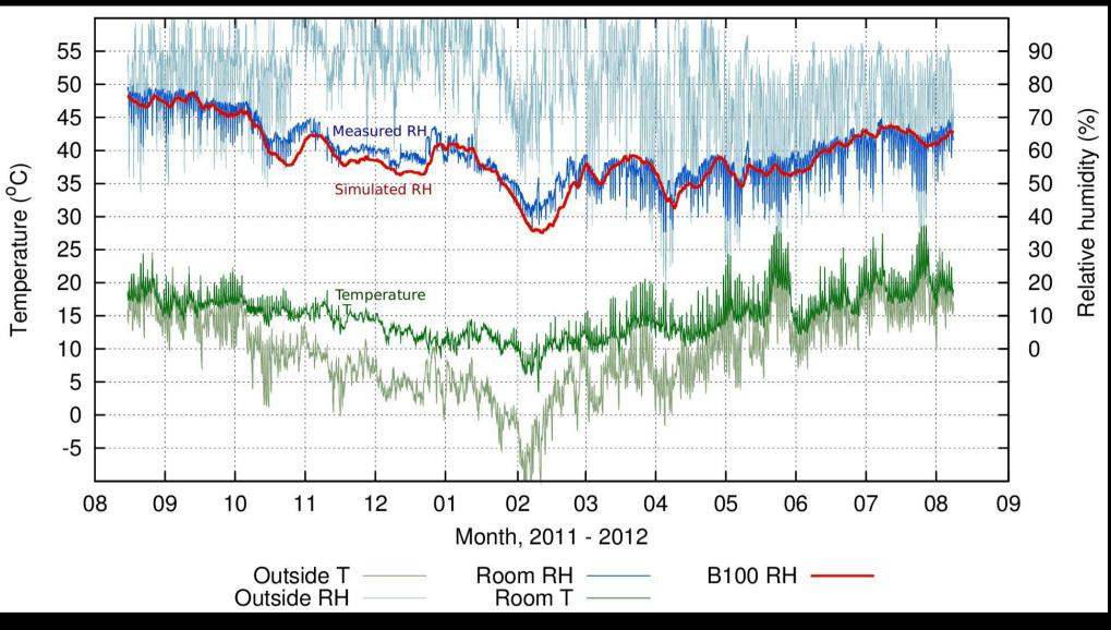
Temperature and RH outside and within the clay lined room. The red trace is the predicted RH. The spikes are due to direct sunlight temporarily overwhelming the buffer capacity of the clay Cool storage is defined within this Published Document as temperatures falling between 5 °C and 18 °C.
