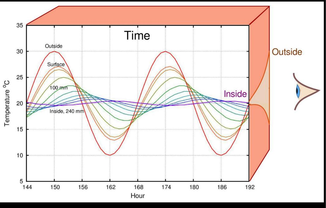
How the daily cycle of temperature penetrates a 240 mm thick solid brick wall
