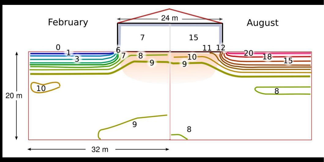
Simulation of the underground temperature contours under a museum store, showing how the ground acts as a huge thermal buffer for the building above
