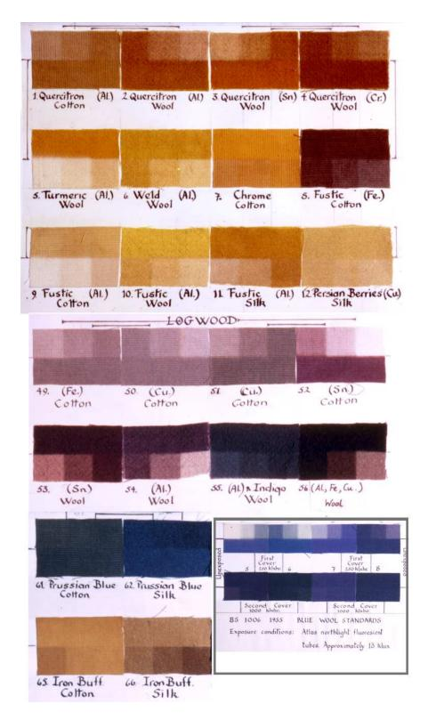
Figure 4: A continuation of figure 1 in the main text. This picture shows more dyes than were displayed (in monochrome) in the original article. The blue wool standards are shown in the inset at bottom right.
