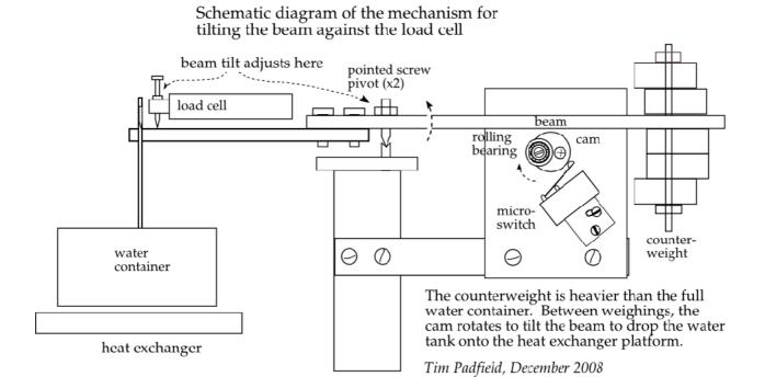
The original bending beam strain gauge has been replaced by a pivoted beam with a load cell registering the out of balance load on the beam.
