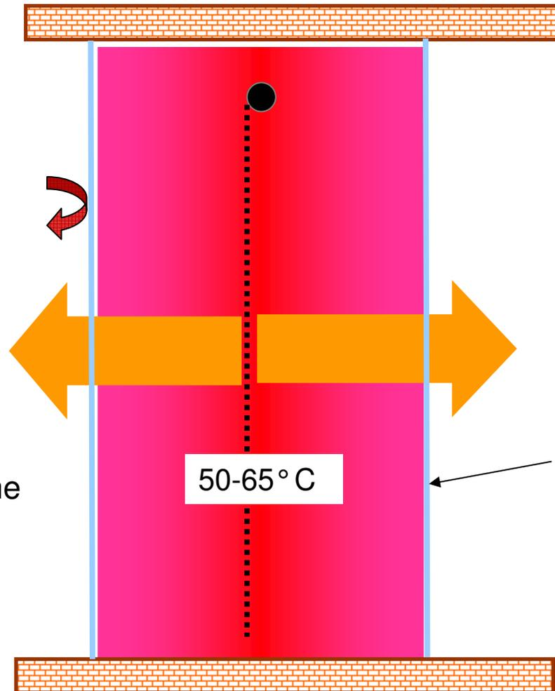
The 1<sup>st</sup> plane of **absorption** emits the highest amount of thermal radiation
