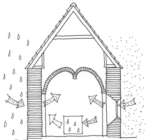
Figure 10. Diagram illustrating the climate control in Karlslunde church. In summer, water vapour is supplied from the outside air through natural ventilation. In winter, water vapour is probably released from the building structure by evaporation. The dehumidifier removes moisture from the interior all year and maintains a constant RH independently of temperature.
