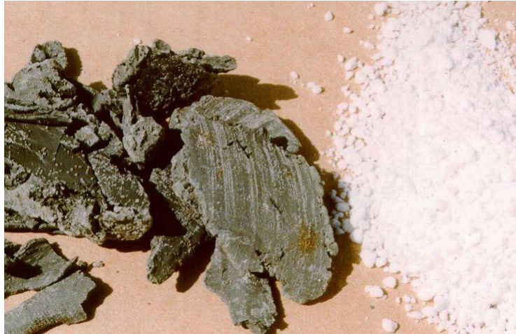
Figure 4.20 Bentonite clay (left) and Perlite grains of up to 2 mm diameter. The bentonite is 80% montmorillonite clay in very finely divided but compact form and is very impermeable indeed. The admixture of perlite opens the structure and makes the resulting tiles dimensionally stable and porous.
