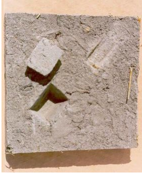
Figure 4.23 A clay tile, 180 mm square, made from bentonite, perlite and straw. A hole was cast into the tile when it was made and a plug was cast to fit the hole. The RH sensor was placed in the hole and the plug was inserted and sealed with moist clay mortar. The shallow hole is for the sensor at the back of the tile. The entire back and the sides of the tile were finally sealed with aluminium foil and polyethylene foil.
