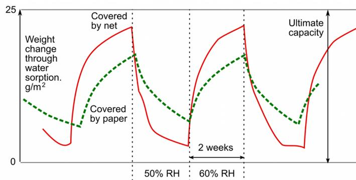
Figure 7: The effect of covering unfired perforated brick with a single layer of filter paper. The response curves to a four week square wave RH cycle are plotted superimposed. The top and bottom boundary lines indicate the ultimate buffer capacity derived from the static sorption measurement. The net had mesh openings 1.2 mm square, the paper was Whatman nr.1, 88 g/m<sup>2</sup>.
