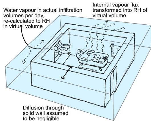
Figure 5: The B-values for all surfaces and furniture, converted to cubic metres, are added to the actual room volume to give a larger, virtual room volume. All water vapour fluxes are led into this volume and then the RH is calculated.
