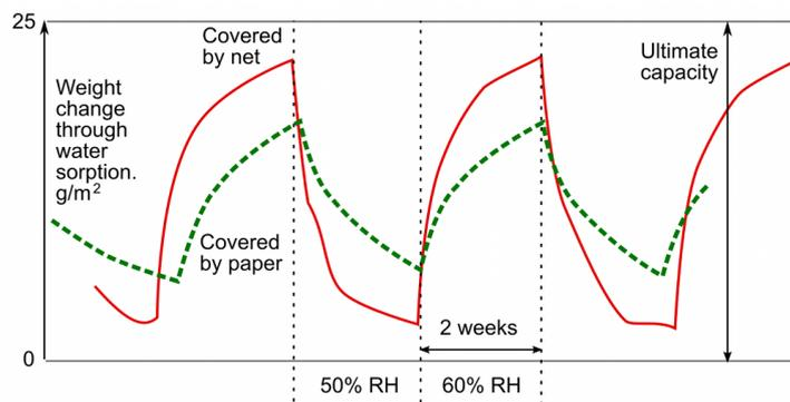
Figure 7: The effect of covering unfired perforated brick with a single layer of filter paper. The response curves to a four week square wave RH cycle are plotted superimposed. The top and bottom boundary lines indicate the ultimate buffer capacity derived from the static sorption measurement. The net had mesh openings 1.2 mm square, the paper was Whatman nr.1, 88 g/m<sup>2</sup>.
