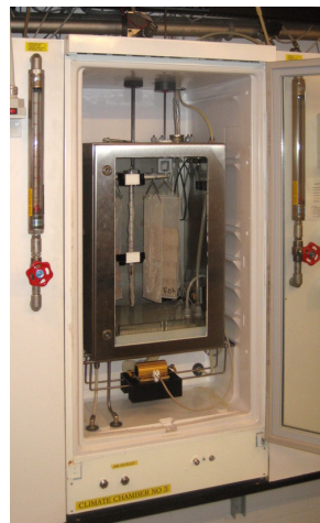
Figure 19: The sorption measuring device. Finely divided specimens are loosely packed in polyester mesh bags which are suspended from a carousel which rotates them in turn to be hooked to a rod, connected via a briefly open tube to a balance mounted out of sight above the picture. The climate is controlled by mixing two air streams, one saturated, the other dry. The entire assembly is held at a constant temperature in a double enclosure.
